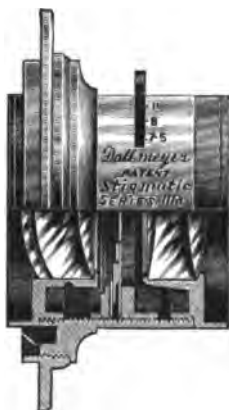
Fig. 103.—Dallmeyer's "Stigmatic." Series IIIa.
